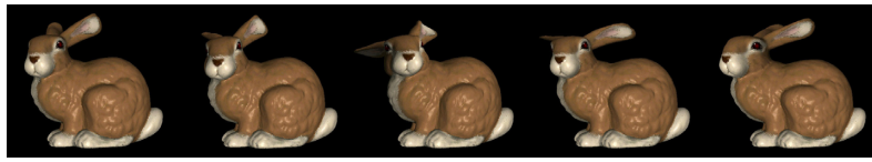
Fig. 1. We swing the head of a point-sampled bunny model with our FFD method.
