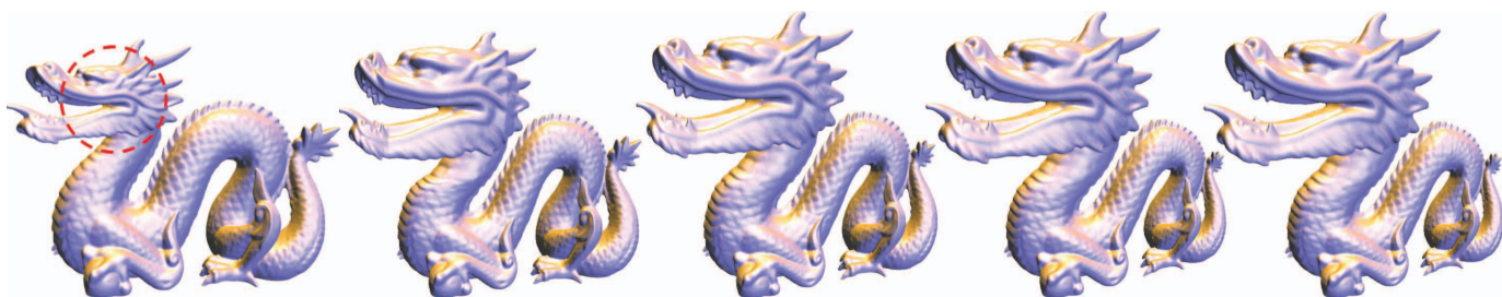
Fig. 6. We magnify the dragon's head (in the red dotted circle) to achieve Focus+Context visualization. From left to right are the original model and the locally magnified models computed by our algorithm after 1, 5, 10, 30 iterations. Notice that the surrounding region of the dragon's head is more distorted in the beginning but the distortion is rapidly reduced in subsequent iterations. The results obtained in 10 and 30 iterations are very similar because the iterative solver has converged.
