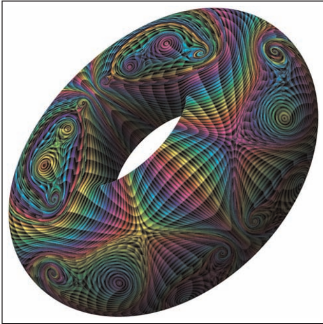
Figure 12. The application of RAPSAs to the visualization of a surface flow synthesized on a 400 \times 400 curvilinear grid of torus. The orthogonal advancing waves help enhance direction cueing as well as depth cueing for a better understanding of the flow movement in 3D settings.
