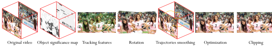
Fig. 3 System overview. First, we must generate a significance map. Then, we track the features in the video. We subsequently remove the shaky turning motion and smooth the trajectories of the features. Next, we perform optimization to obtain a stable video and crop the video with a clipping window.
