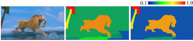
Fig. 3. Significance map generation. Left: input video frame. Middle: significance map. Right: enhanced significance map. Significance values are visualized by colors ranging from blue (lowest significance) to red (highest significance).
