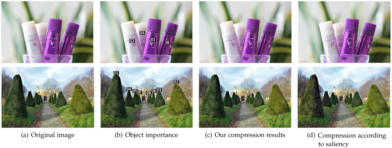
Fig. 17. Adaptive image compression. Our results have better visual quality than those obtained with saliency-based importance information.
