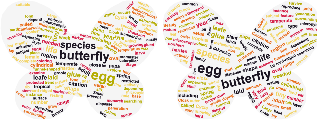
Fig. 6. Demonstration of the use of uniform constraint. Left: word cloud without uniform constraints; right: word cloud with uniform constraints. The gray region represents the specified shape of the layout.
