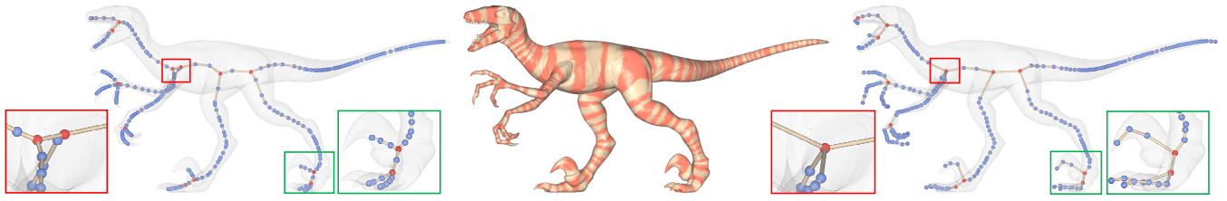
Figure 4: (Left) The 1D structure obtained by performing the connectivity surgery on the contracted mesh in Figure 1. (Middle) The induced skeleton-mesh mapping. (Right) The resulting curve-skeleton after embedding refinement
