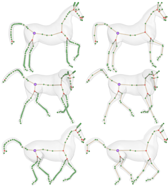
Figure 11: Compatible curve-skeletons (left column) and bone-skeletons (right column) extracted from three poses of a horse model. The root node is drawn in purple.
