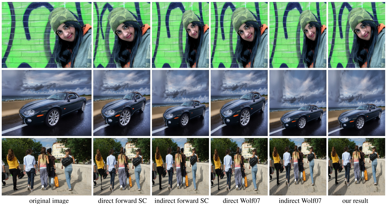
Figure 2: The middle columns present direct and indirect narrowing results by the forward seam carving method [Rubinstein et al. 2008] (denoted as forward SC) and the warping method of [Wolf et al. 2007]. Indirect narrowing achieves the desired aspect ratio by first increasing the height of the image and then downsampling. Note that structural objects, such as the car and jumping people, suffer obvious discontinuity with seam carving. Direct resizing by seam carving preserves the girl’s face but not the car, and indirect resizing preserves the car but not the girl’s face. This is because the homogeneous information is distributed horizontally in the Girl image and vertically in the Car image. For the more complex Walking people image, both previous methods cannot preserve well the aspect ratios of the people with either direct or indirect resizing strategy due to their one-directional propagation of distortion. Our algorithm achieves better results for all three images.
