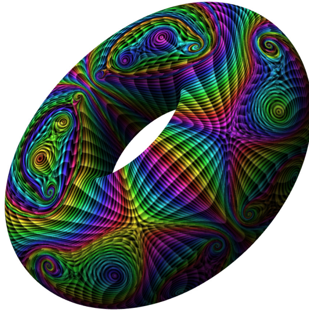
Figure 12. The application of RAPSA to the visualization of a surface flow synthesized on a 400 \times 400 curvilinear grid of torus. The orthogonal advancing waves help enhance direction cueing as well as depth cueing for a better understanding of the flow movement in 3D settings.
